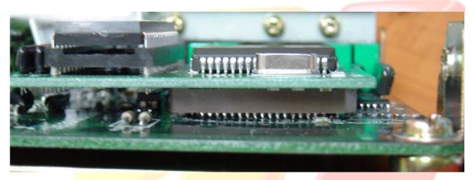
If the right-hand side of this is very slightly lifted higher than the left side (as illustrated in this picture), that's OK. You just want that socket pressed as firmly against the plug as possible.
